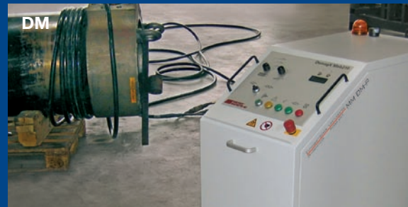
Large individual parts are demagnetized with the DM200 mobile demagnetizer. The flexible cable allows parts to be suitably wrapped in a coil.
