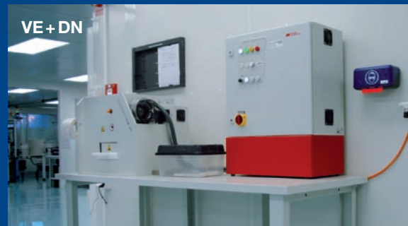
Demagnetization of medical needles by a powerful degaussing pulse. The demagnetization takes about 7 seconds.
