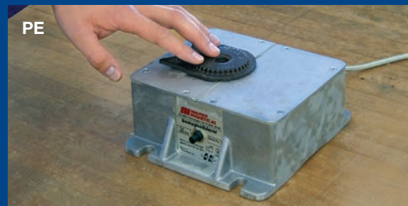
With a classic plate demagnetizer, thin-walled, flat parts are successfully demagnetized.
