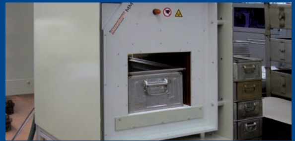
Demagnetization of 500 springs in a 480 x 320 x 210 stainless steel container. The MM VE coil module is equipped with an outer magnetic shield.
