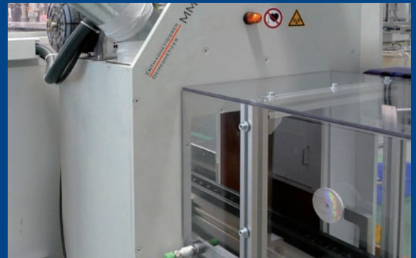
An MM VE with an integrated light barrier for pulse activation, allowing the machine to operate completely automatically.
